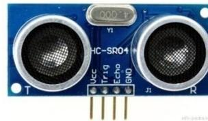
Gambar 1 Sensor ultrasonik HC-SR04
