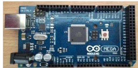
Gambar 2 Papan Arduino MEGA2560
