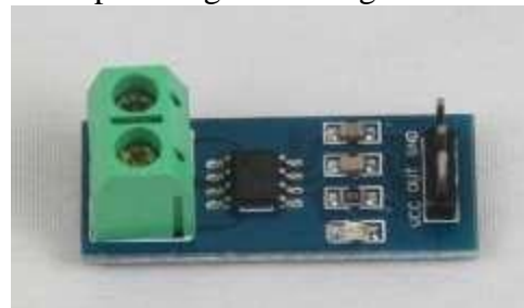
Gambar 8 Sensor Arus ACS 712
